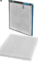
Dynamic Air Cleaners use electronic polarized-media technology for maximum air cleaning capability. Active electronic, polarized-media air cleaners use a safe, 24 volt current to establish a polarized electric field. Airborne particles pass through the field and adhere to the media. The air cleaner's efficiency increases as it loads, providing exceptionally high efficiency with air resistance much lower than expensive disposable filters.
